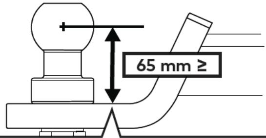
Height from base to center of ball to be 65 mm+
