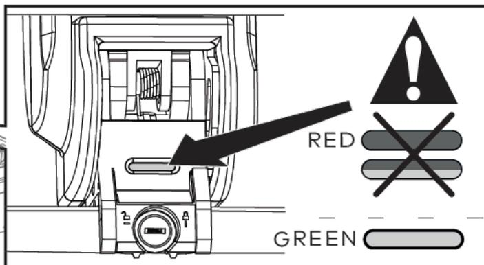
**NOTE** - Ensure the lock is in the unlock position and the indicator window is completely green.
