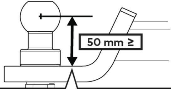
Height from base to center of ball to be 50 mm+
