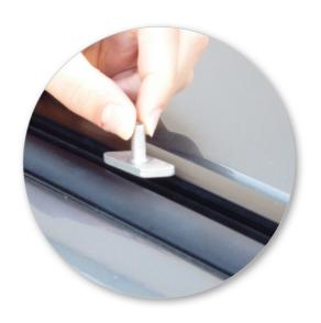
Place T-bolt into track by either inserting it from the top or sliding in from the end.
