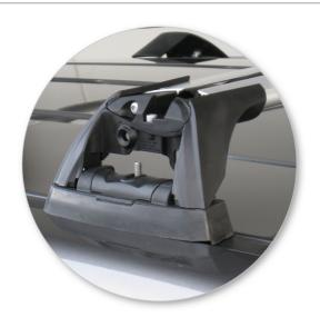
Ensure the pads are in the correct position and the clamp threads pass through the crossbar feet.
