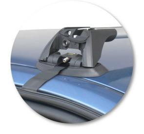
Clamps under rubber door frame mouldings
